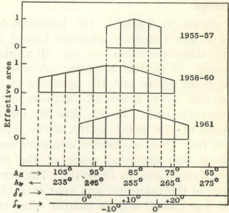
Fig. 6. Azimuthal dependence of the effective area Telescope No. 2.
