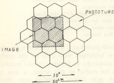
Fig. 2. Arrangement of Phototubes at the Focal Plane and the Image of Cerenkov Light.
