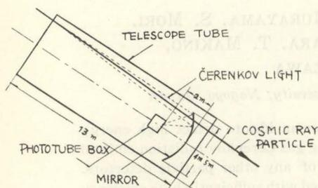
Fig. 1. Principle of the Gas Cerenkov Cosmic-Ray Telescope.
