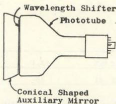
Fig. 6. Conical Shaped Auxiliary Mirror and Wavelength Shifter.
