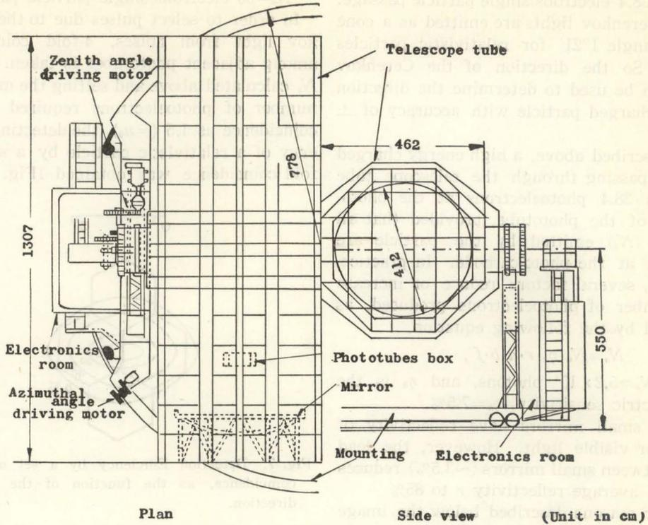
Fig. 4. Telescope Tubes and Alt-Azimuth Mounting.
