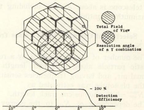
Fig. 9. Total Field of View and the Dependence of Detecting Efficiency to the Direction of the Particle.
