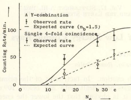
Fig. 10. Counting Rate as the Function of the Total Number of Photoelectrons available at Photocathode,  $N_e$ . a: Phototube only. b. With wavelength shifter. c. Both with wavelength shifter and auxiliary mirror.
