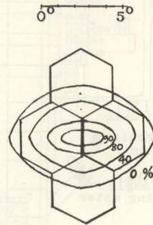
Fig. 7. Detection Efficiency by a set of 4-fold coincidence, as the function of the particle direction.
