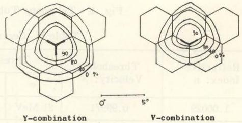
Fig. 8. Detection Efficiency by Combinations of 3 (Y-combination) or 2 (V-combination) sets of 4-fold coincidence.
