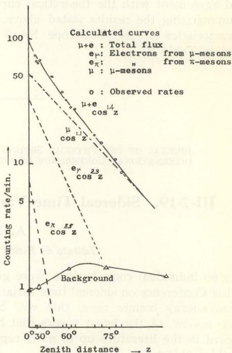
Fig. 11. Zenith Distance Dependence of the Counting Rate of a Y-combination.
