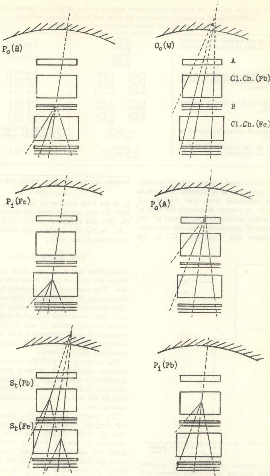
Fig. 2. Schematic illustration of [7] classes of hard showers,  $O_o(W)_{in}$ ,  $P_o(A)$ ,  $P_i(Pb)$ ,  $P_o(B)$ ,  $P_i(Fe)$ ,  $S_t(Pb)$  and  $S_t(Fe)$ .
