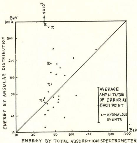
Fig. 3. Plot of primary energy estimated from the angular distribution of the secondaries by the method employed by Castagnoli *et al.* against the energy measured by total absorption spectrometer suitably corrected for unsampled energy losses.
