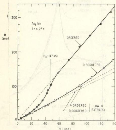
Fig. 3. High magnetic field behavior of  $\text{Au}_3\text{Mn}$  at 4.2°K.
