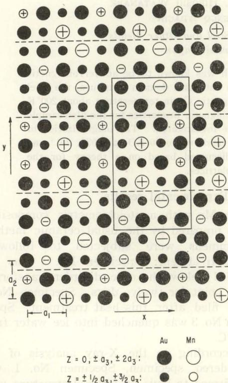
Fig. 4. Idealized orthorhombic superlattice of ordered Au<sub>3</sub>Mn after D. Watanabe, with the moment directions assigned as described in text.
