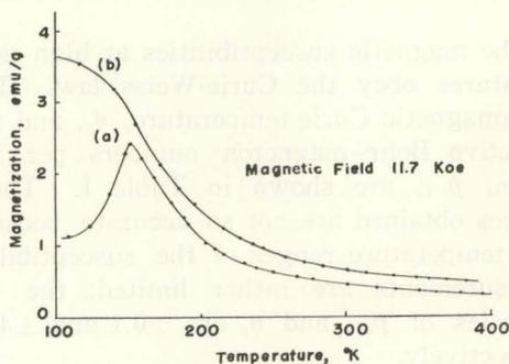
Fig. 6. Magnetization *vs* temperature curves for the  $\alpha'$ -phase specimens of 27% Mn prepared by annealing at (a) 250°C and (b) 100°C.
