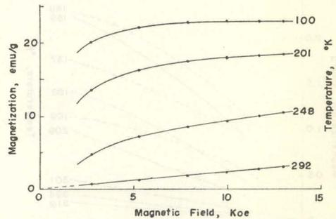
Fig. 2. Magnetization curves for the quenched  $\epsilon$ -phase specimen of 15% Mn.
