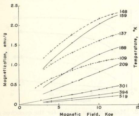
Fig. 4. Magnetization curves for the  $\alpha'$ -phase specimen of 27% Mn prepared by annealing at 250°C (perfectly ordered).
