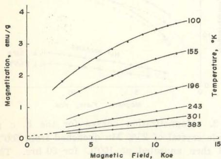
Fig. 5. Magnetization curves for the  $\alpha'$ -phase specimen of 27% Mn prepared by annealing at 100°C (imperfectly ordered).
