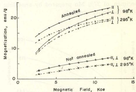
Fig. 3. Magnetization curves for the h. c. p. single crystal of 25% Mn quenched from  $500^\circ\text{C}$  and then annealed at  $100^\circ\text{C}$  for 50 hrs. The measurements were made for both annealed and not-annealed states. The magnetic fields are parallel (||) or perpendicular ( $\perp$ ) to the  $c$ -axis; the temperatures are  $98^\circ$  or  $295^\circ\text{K}$ .
