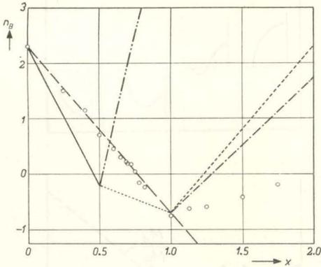
Fig. 3. Saturation moments for the system  $NiFe_{2-x}V_xO_4$ .
