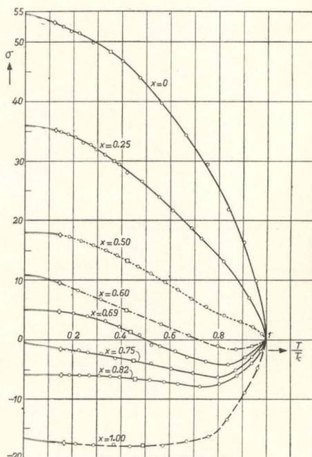
Fig. 1. Saturation magnetization per gram vs reduced temperature for the system  $\text{NiFe}_{2-x}\text{V}_x\text{O}_4$ . ( $0 \leq x \leq 1$ ).
