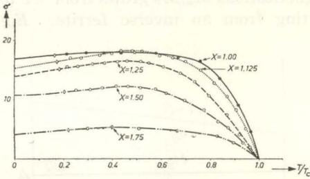
Fig. 2. Saturation magnetization per gram vs reduced temperature for the system  $NiFe_{2-x}V_xO_4$  ( $1 < x < 1.75$ ). For meaning of symbols see Fig. 1.
