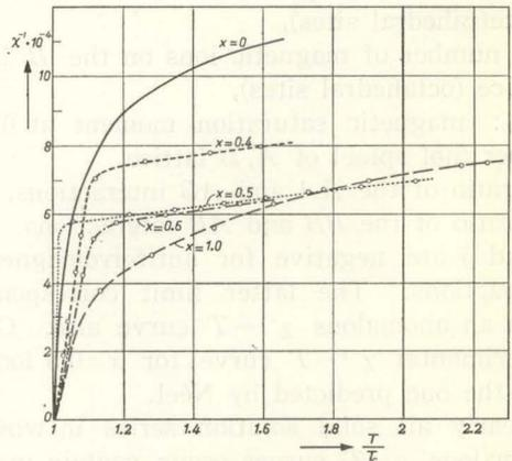
Fig. 5. Reciprocal susceptibility per gram vs reduced temperature for the system  $NiFe_{2-x}V_xO_4$ .
