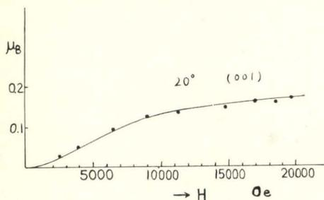
Fig. 4. Magnetization curve in a direction 20° from  $\langle 100 \rangle$  in (001).
