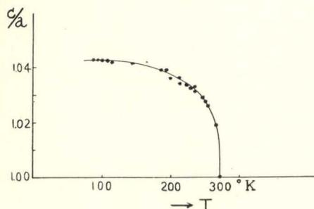
Fig. 2. Temperature dependence of tetragonality of a face-centered unit cell.
