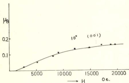
Fig. 3. Magnetization curve in a direction 10° from  $\langle 100 \rangle$  in (001).
