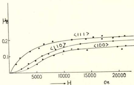
Fig. 5. Magnetization curves for principal axes of a crystal.
