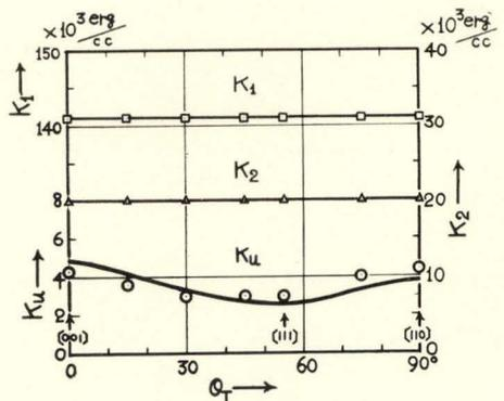
Fig. 4. Dependence of anisotropy constants  $K_1$ ,  $K_2$  and  $K_u$  upon crystallographic direction of the annealing field (17.5 at. % Al-Fe). Circles indicate the experimental results for (110), and the solid line for  $K_u$  was drawn by using  $F=4.9 \times 10^3$  erg/cc and  $G=5.0 \times 10^3$  erg/cc, both values of which were determined by the experiment for (001).
