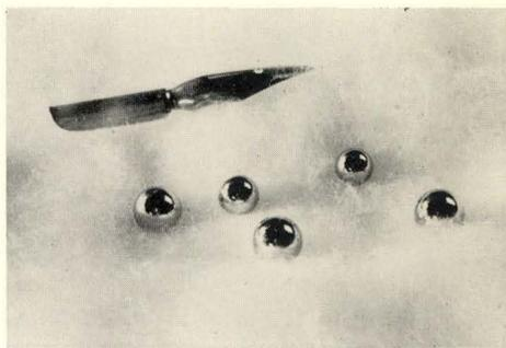
Fig. 1. Single crystal specimens of Fe-Al alloys,
