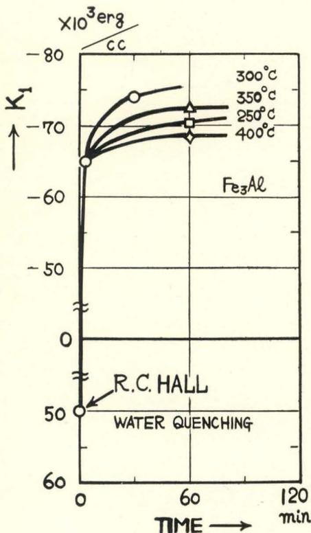
Fig. 3. Change of the magnetocrystalline anisotropy constant  $K_1$  caused by a duration of annealing at various temperatures.
