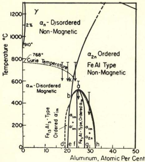
Fig. 2. Phase diagram of Fe-Al system as determined by Taylor and Jones<sup>13)</sup>. Arrows indicate the compositions of the present specimens and temperatures from which the specimens were cooled in a magnetic field.
