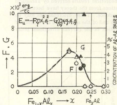
Fig. 5. Dependence of the two coefficients  $F$  (circles) and  $G$  (triangulars) upon the alloy composition of Fe-Al system. Solid marks and hatched marks are due to Suzuki<sup>3)</sup> and Gengnagel and Wagner<sup>9)</sup> respectively. The broken line indicates the number of Al-Al pairs as determined by Biorci, Ferro and Montalenti<sup>7)</sup> by using the x-ray data of Bradley and Jay<sup>10)</sup>.
