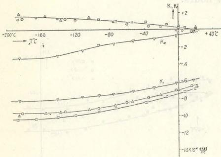
Fig. 2. The anisotropy constants,  $K_1$  and  $K_2$ , vs temperature.
