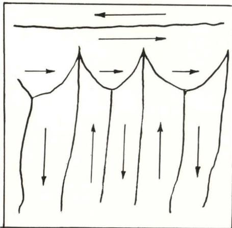
Fig. 7. c. Domain structure of the edge zone of an iron film ( $\times 600$ ).
