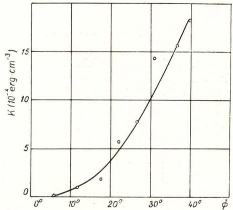
Fig. 5. Dependence of constant of uniaxial magnetic anisotropy on the incidence angle for iron films deposited on glass substrate kept at 100°C, without using the rotating diaphragm.
