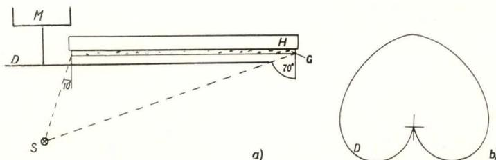
Fig. 2. a) Diagram of deposition arrangement; S denotes source of evaporation, D rotating diaphragm, G glass substrate, H heater, M motor.
