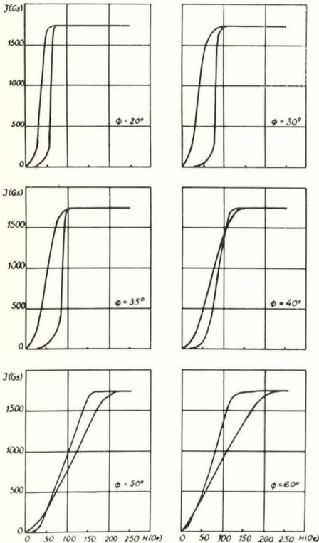
Fig. 4. Initial magnetisation curves for different incidence angles, measured in the direction of the easy axis and perpendicular to it.
