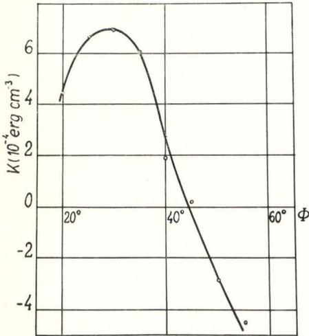
Fig. 3. Dependence of constant of uniaxial magnetic anisotropy on the incidence angle for iron film deposited on glass substrate kept at 100°C using the rotating diaphragm.
