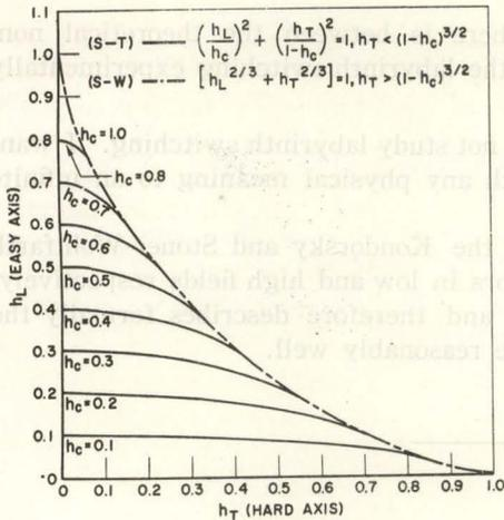
Fig. 4. Theoretical critical switching curves, for several values of the reduced coercive force  $h_c$ , derived from the Shtrikman and Treves (S-T) model. Also the critical curve derived from the Stoner and Wohlfarth (S-W) model to which the (S-T) model reduces when  $h_T = (1-h_c)^{3/2}$ .
