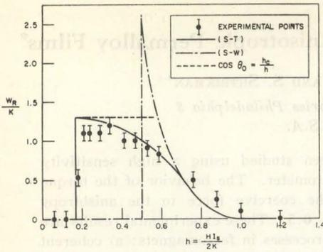
Fig. 2. Rotational hysteresis  $W_r$ , plotted in reduced units, vs. reduced applied field. The theoretical curves are those derived from the treatments by Shtrikman and Treves (S-T), Stoner and Wohlfarth (S-W), and Kondorsky.
