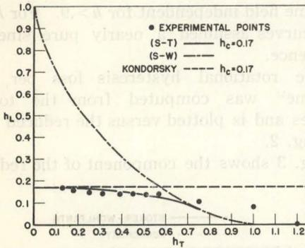
Fig. 3. The component of the reduced critical field in the easy direction,  $h_L$ , vs. the component in the hard direction  $h_T$ . The theoretical curves are those derived from the treatments by Shtrikman and Treves (S-T), Stoner and Wohlfarth (S-W), and Kondorsky.
