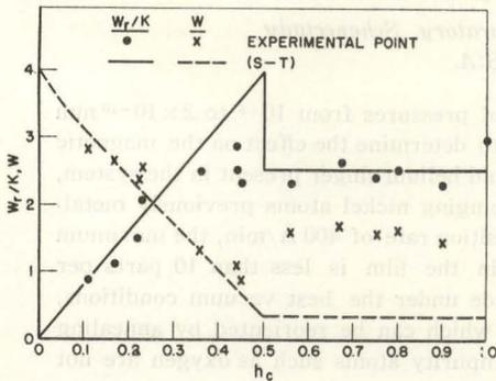
Fig. 5. The dependence of the maximum reduced rotational hysteresis  $W_r/K$  and the rotational hysteresis integral  $W$  on the reduced coercive force  $h_c$ . The theoretical curves are derived from the Shtrikman and Treves (S-T) model which reduces to the Stoner and Wohlfarth (S-W) model for  $h_c > 0.5$ .
