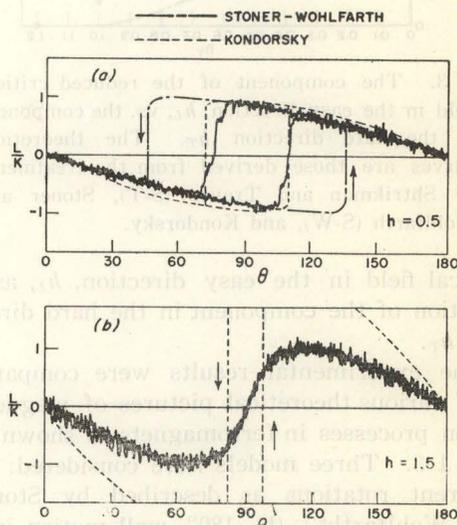
Fig. 1. Angular dependence of the torque  $L$ , plotted in reduced units, for two values of the reduced applied field; (a)  $h = 0.5$ , (b)  $h = 1.5$ . The broken curves are those calculated from the Stoner-Wohlfarth (S-W) and Kondorsky models. Reversible portions of the (S-W) curves are not shown in both (a) and (b), since they fall on the experimental curves. Arrows indicate the direction of rotation of  $h$ .
