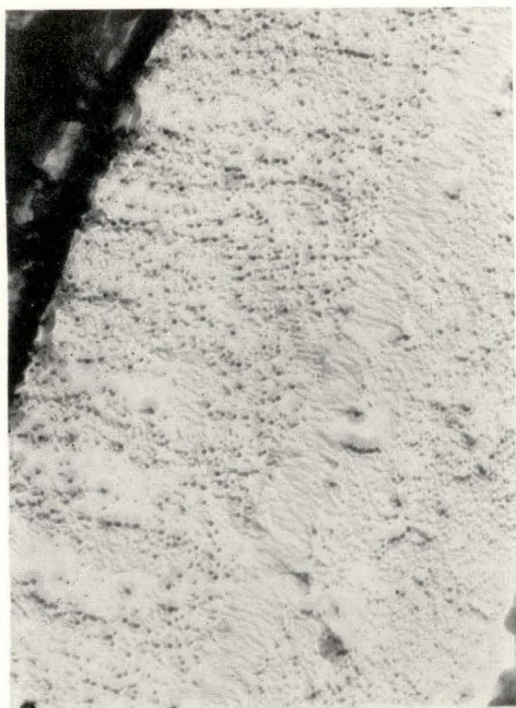
Fig. 4. Cross section electron micrograph showing evidence for the columnar growth in the central portion of the picture and the lines of etch pits toward the substrate marking the high energy regions of the film.
