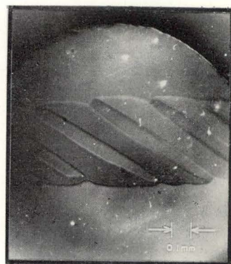
Fig. 3. "Candy-Cane" Domain—a combination of easy direction domains and those at 45^\circ to the easy direction as viewed with analyzer and polarizer near extinction and the easy axis parallel to the page horizontal.
