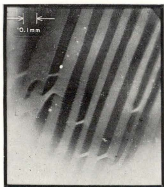
Fig. 2. Bar Domains at about 45^\circ to the easy direction showing cross-ties and magnetization ripple.
