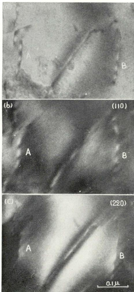
Fig. 9. Complex dotted image due to multiple reflections.
