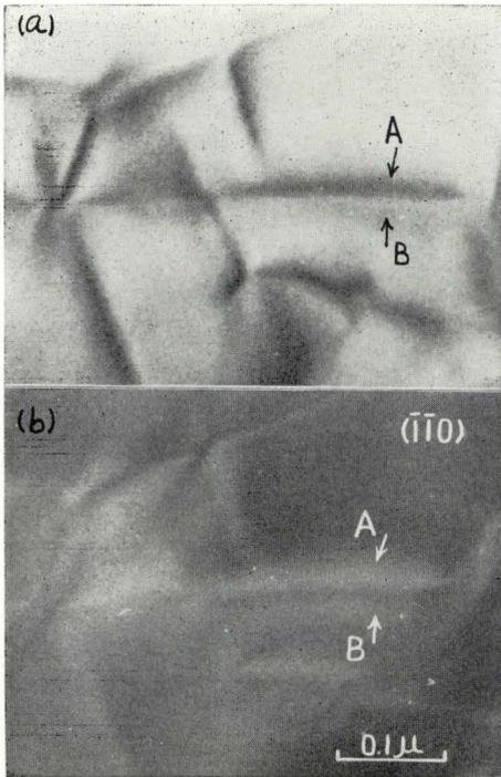
Fig. 3. Double image produced by a single reflection.
