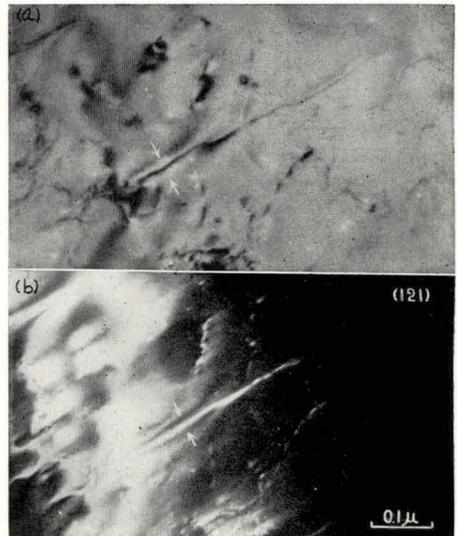
Fig. 1. Single image of dislocation produced by one reflection.
