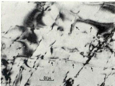
Fig. 12. Extinction contour due to the local bending.
