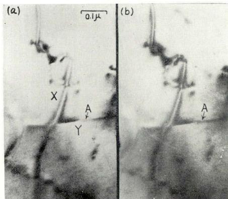
Fig. 11. Reversal of image contrast and double image at the intersecting dislocations.
