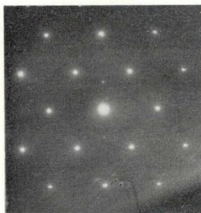
Photo. 7. Electron diffraction pattern corresponding to Photo. 6. The diffraction spots are due to f.c.c. crystal.
