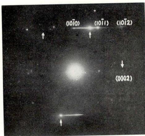
Photo. 2. Electron diffraction pattern corresponding to the specimen in Photo. 1. Diffraction spots due to f.c.c. crystal are indicated by arrows.
