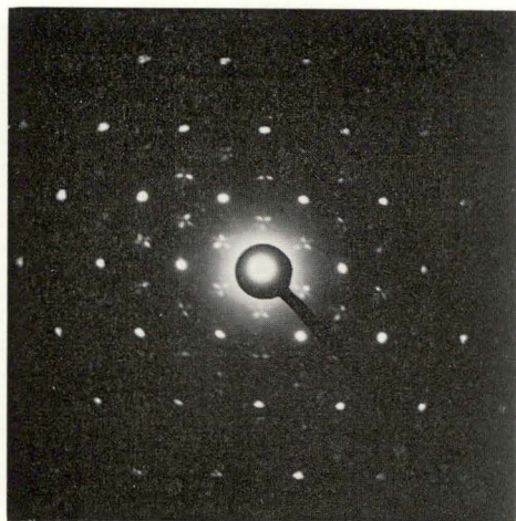
Fig. 2. Electron diffraction pattern of \text{U}_3\text{O}_{8-x} obtained by reduction of the sample of Fig. 1. The spot splitting becomes more pronounced as the reduction proceeds further.
