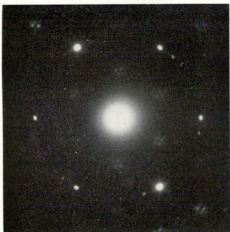
Fig. 4. Electron diffraction pattern of U_3O_{8-x} showing split spots and satellites. Enlarged about twice as compared with Figs. 1 and 2.
