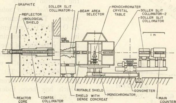
Fig. 2. Vertical drawing of the diffractometer.
