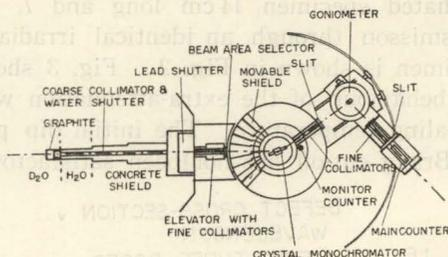
Fig. 1. Horizontal drawing of the diffractometer.
