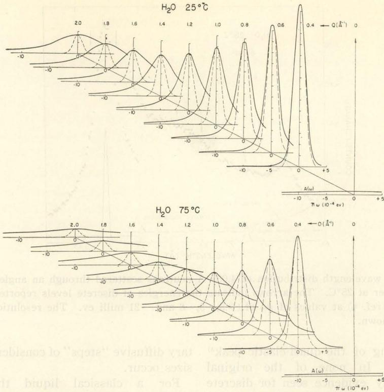
Fig. 1. The scattering function  $S(Q, \omega)$  for water (a) at 25°C and (b) at 75°C for small values of  $\hbar\omega$ . The energy resolution functions are shown as dashed curves. The multiple scattering  $A(\omega)$  which was subtracted is also shown.
