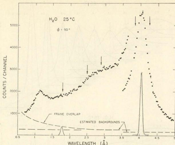
Fig. 3. The wavelength distribution of 4.059 Å neutrons scattered through an angle of  $90^\circ$  by light water at  $25^\circ\text{C}$ . The arrows indicate the energies of discrete levels reported by other workers (ref. 4) at values of  $\hbar\omega$  of  $\pm 0.5, -5, -8$  and  $-21$  milli ev. The resolution function is also shown.
