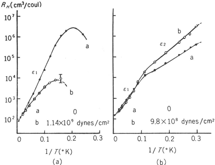
Fig. 2. (a) Hall coefficient with and without stress in arsenic-doped germanium of concentration  $8.3\times 10^{16}$  cm<sup>-3</sup>. (b) Hall coefficient with and without stress in antimony-doped germanium of  $5.0\times 10^{16}$  cm<sup>-3</sup>.
