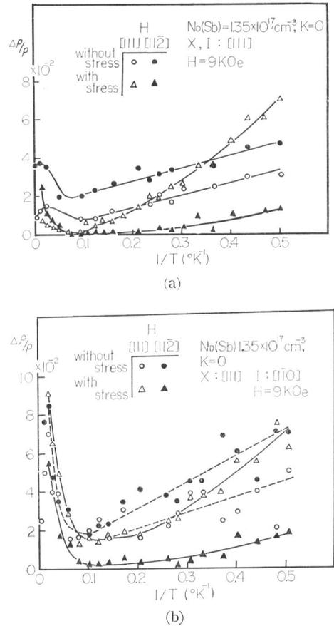
Fig. 5. (a) Longitudinal magnetoresistance in [111] direction in the same sample as that of Fig. 4. Stress  $10^9$  dynes/cm<sup>2</sup>. (b) Transverse magnetoresistance in [110] current direction.
