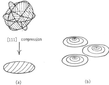
Fig. 3. (a) Ground state wave function made of four pancake-like wave functions is modified by shear strains resulting in one pancake-like wave function originating from [111] valley. (b) Pancake-like wave functions cause anisotropy of overlap.
