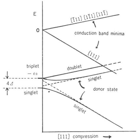
Fig. 1. Energy diagram of the valleys of the conduction band and of the 1s-like levels of group V donor as a function of [111] compression.
