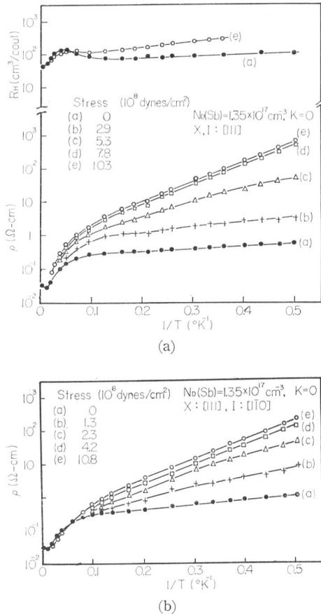
Fig. 4. (a) Piezoresistance in [111] direction under [111] compression in antimony-doped germanium of concentration  $1.35 \times 10^{17}$  cm<sup>-3</sup>. (b) Piezoresistance in [110] direction under [111] compression in the same sample.
