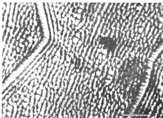
Fig. 3. Last stage of ion etching for MoS 2 .
