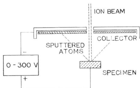
Fig. 1. Experimental arrangement showing specimen and collector.
