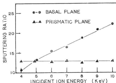
Fig. 5. Sputtering ratios vs incident ion energy. Probable error in the measurements of sputtering ratios is about  $\pm 1$ .
