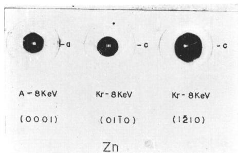
Fig. 2. Sputtering deposit patterns from various planes of zinc crystal. (Faint thorn-like figures which may be visible along the peripheries of deposit patterns are the trace of meshes of section paper used as the background of the picture. They have nothing to do with the deposit patterns, of course.)
