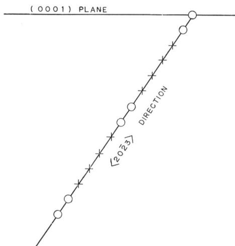
Fig. 6. Atomic arrangement in  $\langle 20\bar{2}3 \rangle$  direction in zinc crystal.
