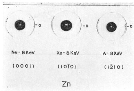
Fig. 3. Sputtering deposit patterns from various planes of zinc crystal. (Faint thorn-like figures which may be visible along the peripheries of deposit patterns are the trace of meshes of section paper used as the background of the picture. They have nothing to do with the deposit patterns, of course.)
