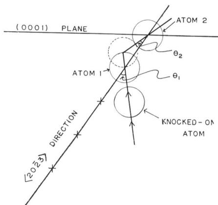
Fig. 7. "Single event focusing" in  $\langle 20\bar{2}3 \rangle$  direction in zinc crystal.
