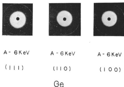
Fig. 4. Sputtering deposit patterns from various planes of germanium crystal.
