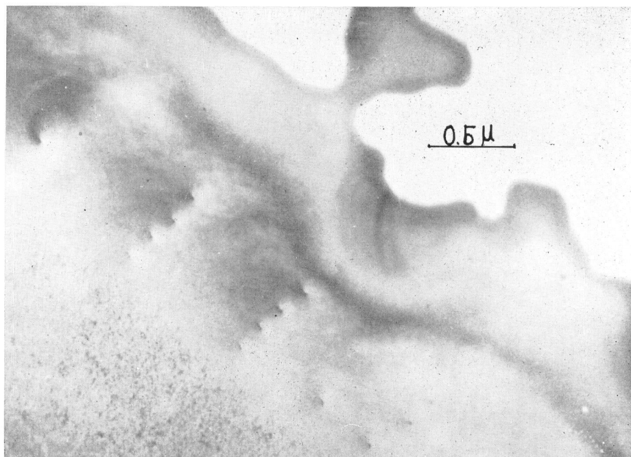
Fig. 1. A transmission electron micrograph of a clean thin sodium chloride single crystal film prepared by the method in the text. Note the arrays of dislocations introduced by bending the crystal before thinning.
