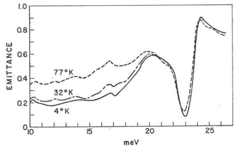
Fig. 1. Spectral emittance of indium antimonide at 4.2, 32, and 77°K. Sample was *n*-type 1.23 millimeters thick having a carrier concentration of  $7 \times 10^{13} \text{ cc}^{-1}$ .
