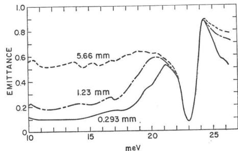
Fig. 2. Spectral emittance of *n*-type indium antimonide at 4.2°K for sample thicknesses of 0.293, 1.23, and 5.66 millimeters. Carrier concentration was  $7 \times 10^{13} \text{ cc}^{-1}$ .
