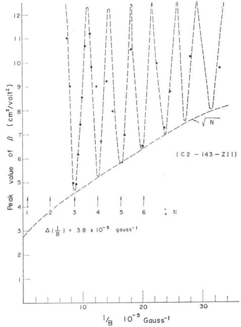
Fig. 5. The oscillatory curves of  $\beta_{\text{peak}}$  as a function of  $1/B$ . This figure is replotted from Fig. 4.
