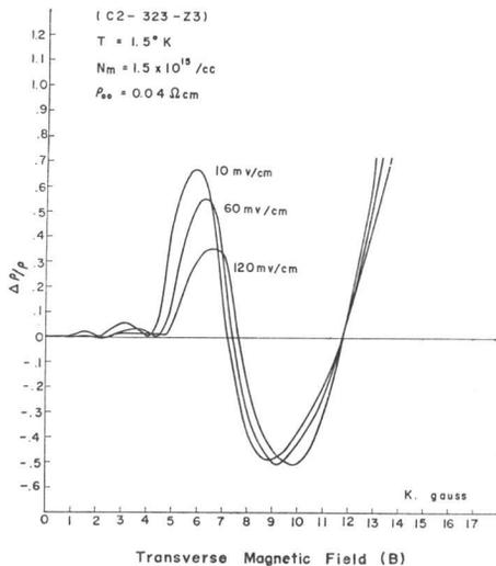
Fig. 2.  $\Delta\rho/\rho$  vs. transverse magnetic field, with electric field as a parameter.
