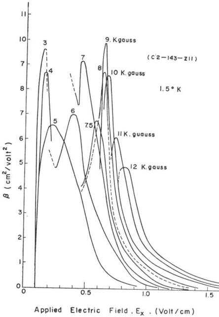
Fig. 4. The change of  $\beta$  as a function of  $E_x$ ; curves are plotted for several magnetic fields.
