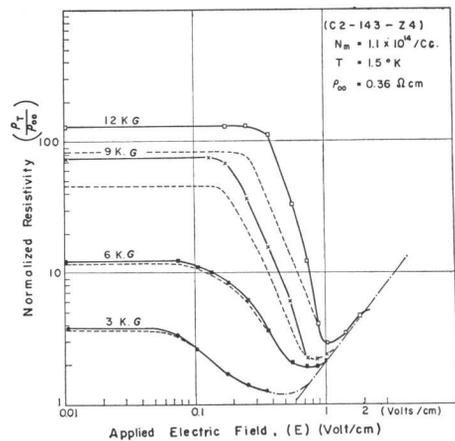
Fig. 1.  $\rho_T/\rho_{00}$  vs. applied electric field for an *n*-InSb sample with an impurity concentration of  $1.1 \times 10^{14}/\text{cc}$ . Freeze-out effect is corrected by dots.
