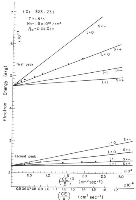
Fig. 3. The shift of electron energy in the magnetic sub-bands as a function of  $(cE_t/B)$ .
