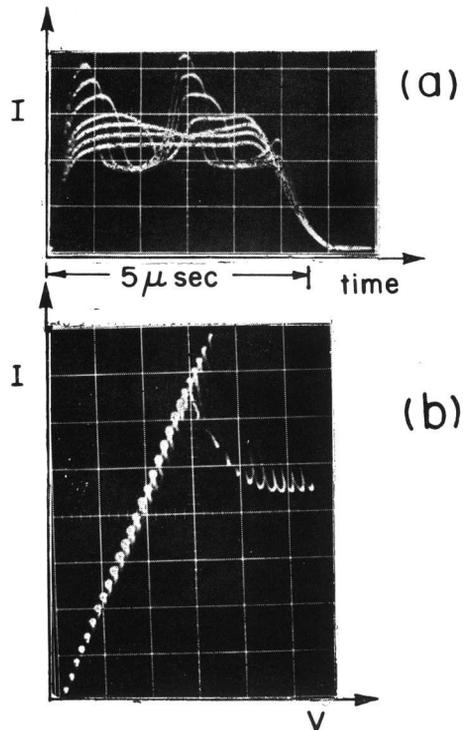
Fig. 1. (a) Current oscillation patterns. (b) Current-voltage characteristic. Li-diffused *p*-GaSb at 77°K; hole concentration =  $8.2 \times 10^{15}/\text{cm}^3$ ; mobility =  $3280 \text{ cm}^2/\text{V sec}$ .
