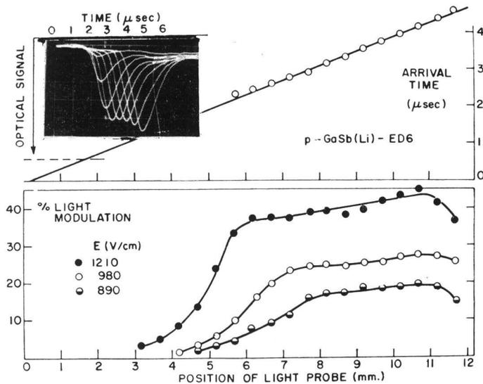
Fig. 2. Results of optical probe study. Li-diffused  $p$ -GaSb at  $77^\circ\text{K}$ . Resistivity =  $1 \Omega \cdot \text{cm}$ . Inset: Oscilloscope traces of optical modulation signals at various positions on the sample. Upper figure: Arrival time of domain peak as a function of position along the sample. Lower figure: Magnitude of modulation signal as a function of position, for several voltages.
