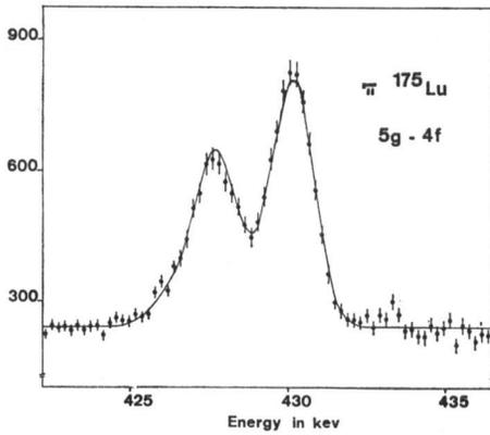
Fig. 1. Energy spectrum of  $5g - 4f$  transition in  $\pi^{175}\text{Lu}$ , obtained with a 1 cc planar Ge(Li) detector. The total number of counts is given as a function of the energy.
