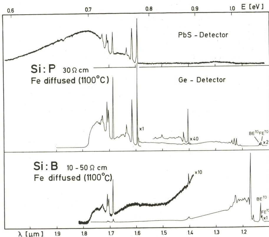
Fig.1 Photoluminescence spectra of Fe-doped silicon:
