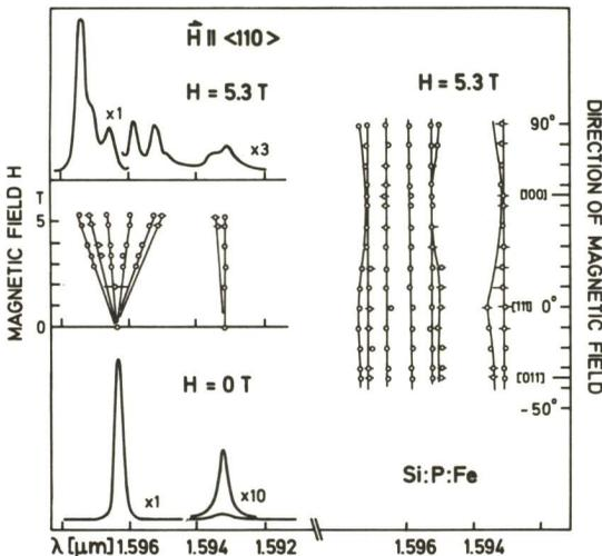
Fig. 2 Zeeman-splitting and angular dependence of the zero phonon lines at 1.6 μm
