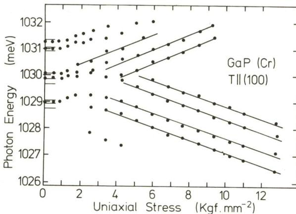
FIGURE 6 the uniaxial stress dependence for compressive stress  $T \parallel (100)$ : The lines moving to higher energies disappear due to thermalization
