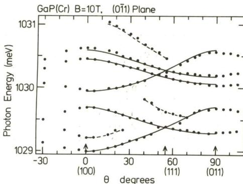
FIGURE 3 the Zeeman anisotropy at 10 T with  $B$  rotated in the  $(0\bar{1}1)$  plane: The data points agree well with the predictions of a simple  $(100)$  axial defect model (solid lines). See also Figure (4)
