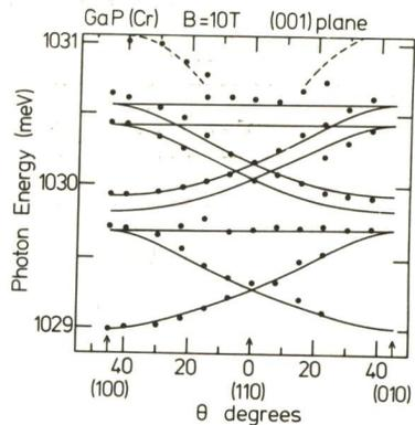
FIGURE 4 the Zeeman anisotropy at 10 T with  $B$  rotated in the  $(001)$  plane
