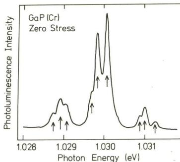
FIGURE 1 the zero phonon fine structure in the PL spectrum of GaP(Cr) at 2 K (zero magnetic field and zero uniaxial stress)
