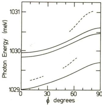
FIGURE 5 variation of the recombination energy as a function of  $\phi$ , the angle between  $B$  and the principal axis of the defect: The curves are deduced from the data points in Figure (3)
