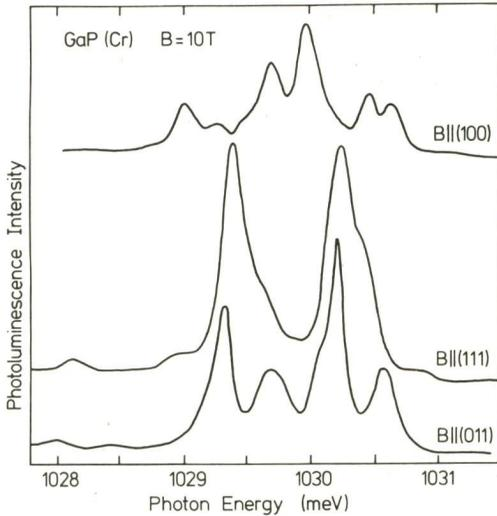
FIGURE 2 the Zeeman-split zero phonon system at 10 T with  $B$  parallel to the three principal axes
