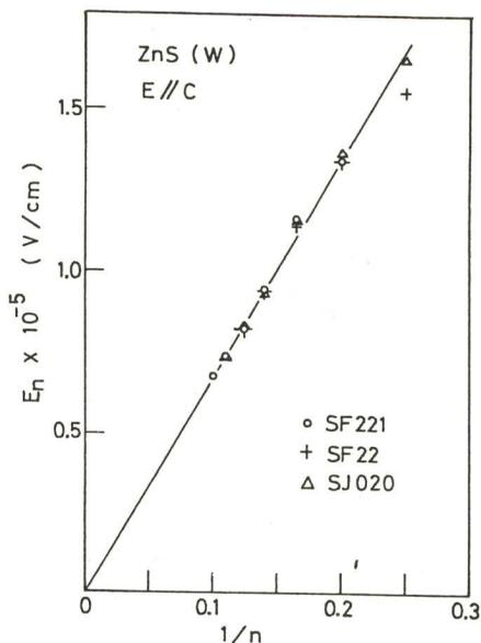
Fig. 3. Linear dependence of the critical field  $E_n$  on  $1/n$
