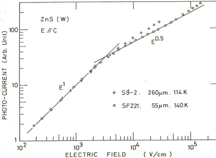
Fig. 1. Photo-current vs electric field characteristics of ZnS along c-axis
