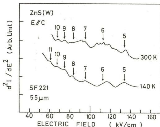
Fig. 2. Oscillation of the second derivatives of the current as a function of the field
