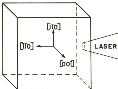
Fig. (1) Experimental configuration for the infrared imaging experiment: A continuous, focused laser beam produces a cloud of EHD. Thermalization phonons are also produced near the excitation point which push droplets into the crystal
