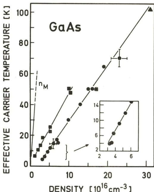
Fig. (3) Density of the EHP at different temperatures: The ● represent data from transmission experiments and the ■ stand for gain measurements. ▲ was derived from the Raman spectrum of Fig.(2)
