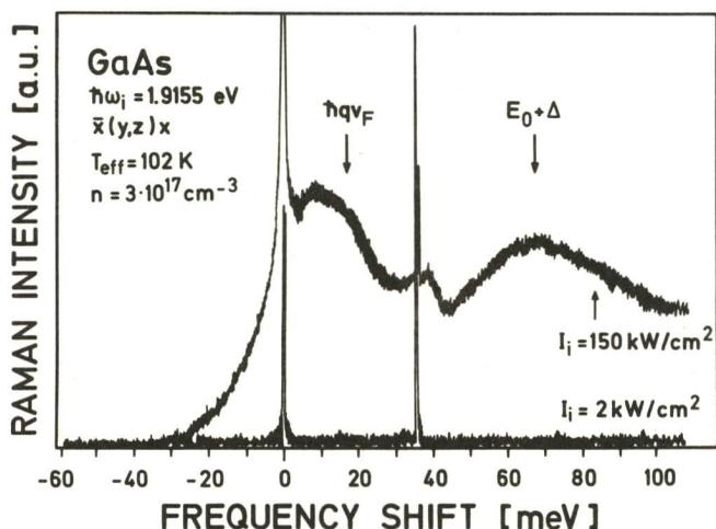
Fig. (2) Raman scattering from an optically excited EHP in backscattering geometry on a (100) surface
