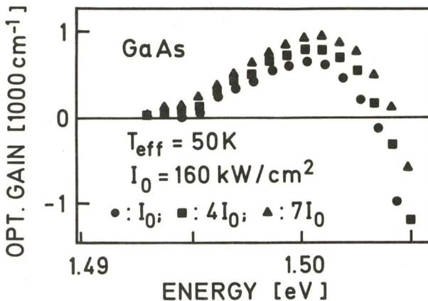
Fig.(1) Optical gain spectra of GaAs as obtained with a two laser transmission experiment at a carrier temperature of 50 K and at three different excitation intensities
