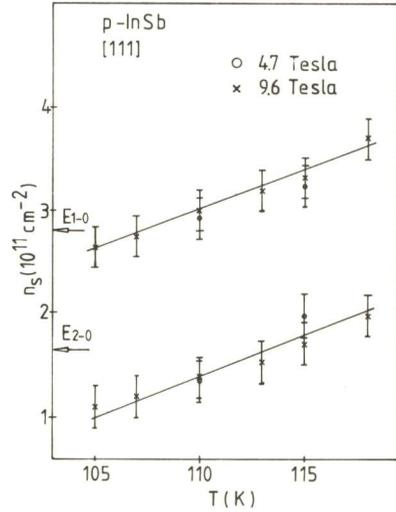
Fig.(3) Temperature dependence of the  $n_S$  values of the electro-phonon resonances: The arrows denote the  $n_S$  values at which  $E_{n-o} = \hbar\omega_{LO}$  at  $S_B=0$  [3,4]
