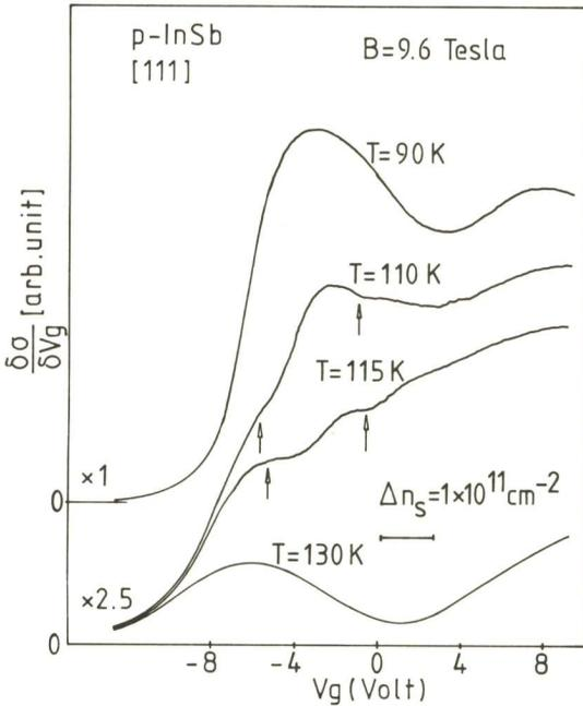
Fig.(2) Transconductance versus gate voltage at a high magnetic field  $B$ : The arrows indicate the newly observed structures
