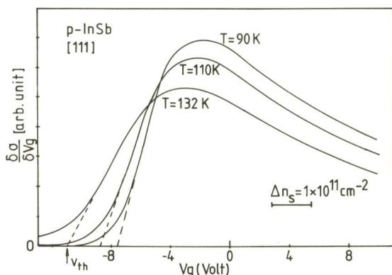
Fig.(1) Transconductance versus gate voltage for elevated temperatures at  $B=0$ : The peak mobility at  $90\text{K}$  is  $\mu_{FE} = 4.9 \times 10^4 \text{ cm}^2/\text{Vsec}$
