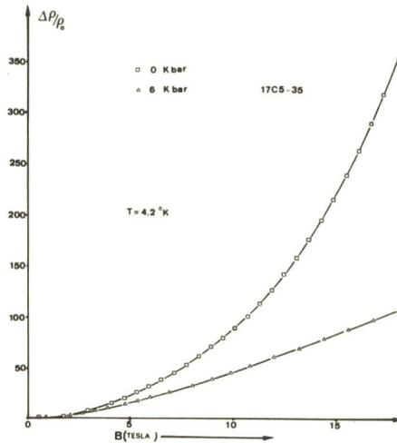
Figure 6 shows the evolution of the SdH oscillation as a function of the hydrostatic pressure at 4.2K. A change in the periodicity of the oscillations could be observed. If we take a pressure coefficient of 9meV/Kbar [13], [14] for two different pressures  $P_1$  and  $P_2$ , then
