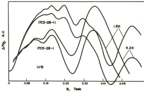
Fig.3 Longitudinal magnetoresistance of different samples at 1.8K and 4.2K
