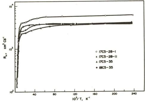
Fig.2 Hall coefficient vs reciprocal temperature
