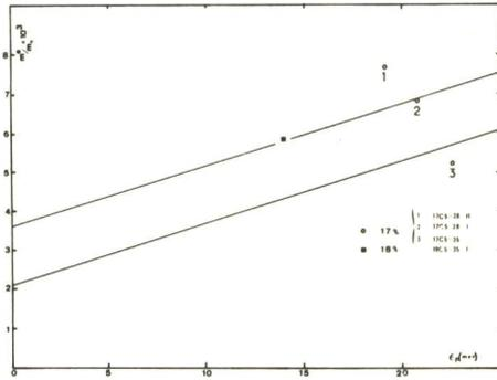
Fig.5 Electron effective mass  $m^*(E_F)/m_0$  vs Fermi level; Straight lines are  $m^*(E_F) = m_0(1 + \frac{3E_F}{E_g})$  for  $x = 0.17$  and  $0.18$ .
