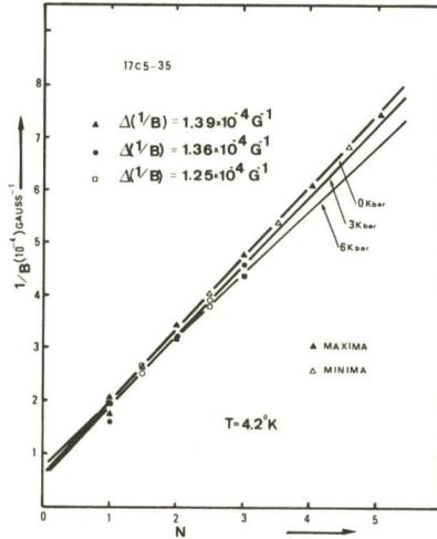
Fig.6 SdH oscillation periodicity as a function of the pressure
