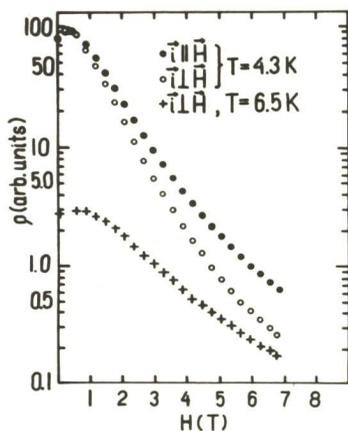
Fig.1 Resistivity versus magnetic field for a sample with  $x \approx 0.155$
