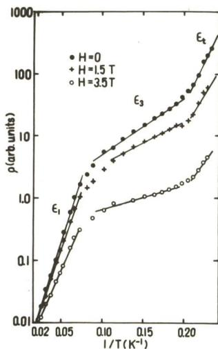
Fig.2 Transverse resistivity versus inverse temperature for a sample with  $x \approx 0.155$ : The activation energies corresponding to the three temperature ranges are indicated
