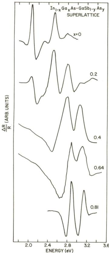
Fig. 2 Room-temperature electroreflectance spectra of various  $\text{In}_{1-x}\text{Ga}_x\text{As}-\text{GaSb}_{1-y}\text{As}_y$  superlattices
