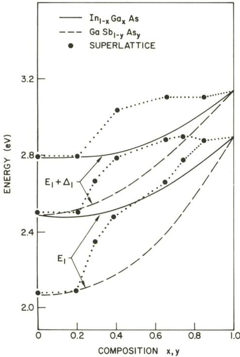
Fig. 3 Variation of the  $E_1$  and  $E_1 + \Delta_1$  transitions with composition for  $\text{In}_{1-x}\text{Ga}_x\text{As-GaSb}_{1-y}\text{As}_y$  superlattices and for the  $\text{In}_{1-x}\text{Ga}_x\text{As}$  and  $\text{GaSb}_{1-y}\text{As}_y$  systems
