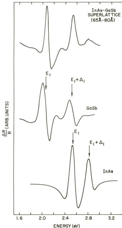
Fig. 1 Room-temperature electroreflectance spectra of InAs-GaSb superlattice and bulk GaSb and InAs
