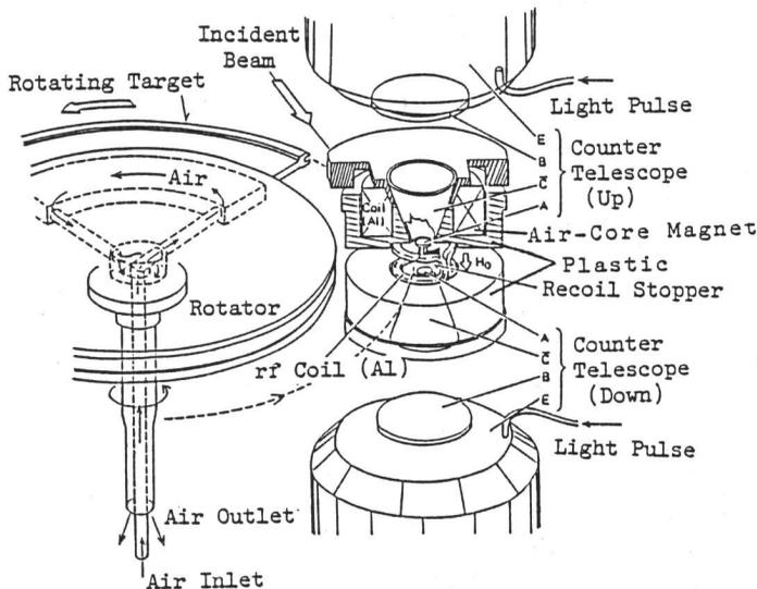
Fig. 1. Experimental setup. The principal part of the chamber wall is made of plastic. Details are given in the text. The metallic target evaporated on a molybdenum ribbon was mounted in the groove of the target holder which is cooled by a jet of air. The rotating wheel was rotated at a period of 60 msec. During the counting time the target with unwanted  $\beta$  emitters were hidden in the radiation shielded area.
