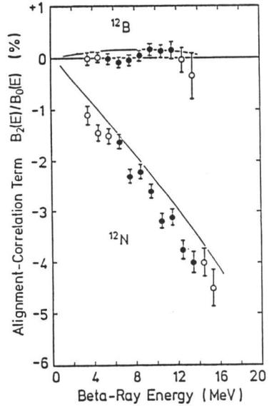
Fig. 3. Alignment-correlation terms for  $^{12}\text{B}$  and  $^{12}\text{N}$ .
