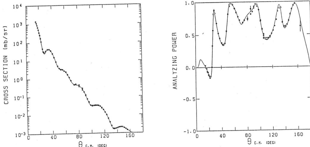
Fig. 1  $^{40}\text{Ca}(p,p)^{40}\text{Ca}$  cross sections and analyzing powers. Solid curves are Fourier-Bessel type optical potential calculations.
