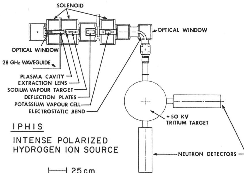
Fig. 1. Layout of the TRIUMF optically pumped ion source with scattering chamber for polarization measurements.
