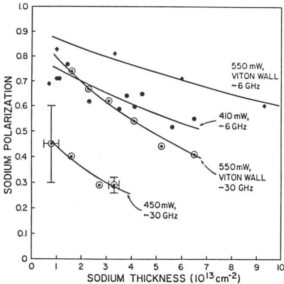
Fig. 2. Measured polarization of a sodium vapour target vs. the target thickness for optical pumping with ~30 GHz and ~6 GHz bandwidth at the sodium D1 line with and without a Viton wall liner.
