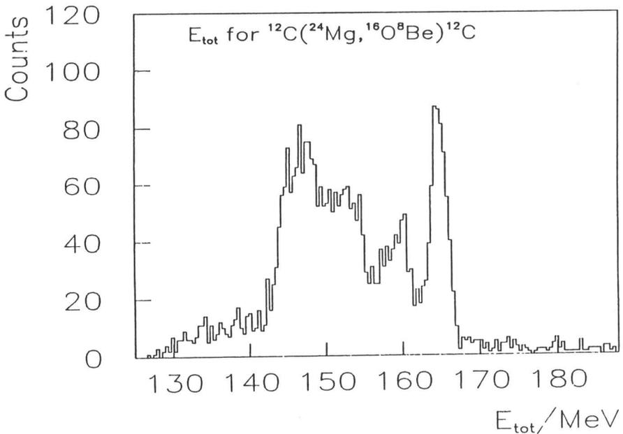
Figure 4 shows the  $E_{\text{tot}}$  spectrum for coincident 160 and  $^8\text{Be}$  nuclei detected in the telescopes. The peaks visible in this spectrum imply a three body
