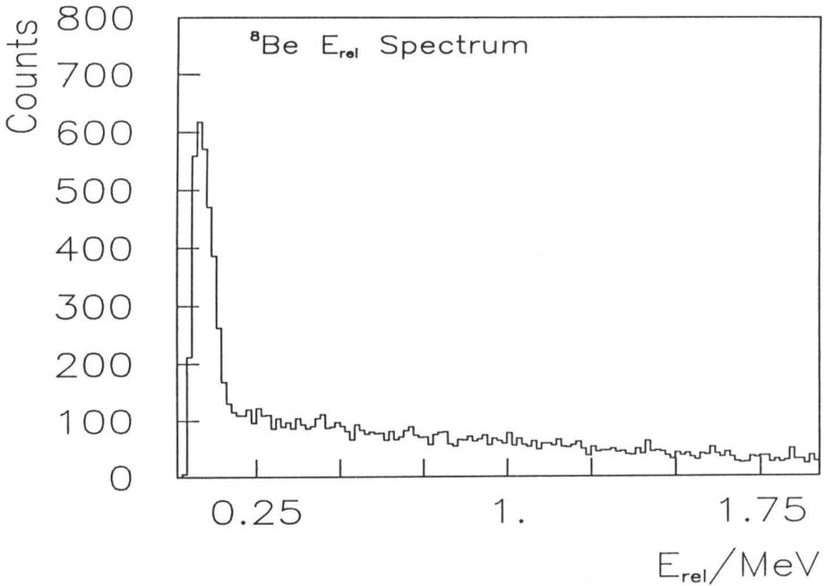
Figure 3 shows an Erel spectrum for events in this detector with a peak visible at the low energy end of the spectrum from decays of  $^8\text{Be}$  nuclei.
