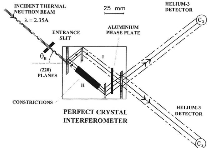
Fig. 2. Schematic of the expected experimental arrangement showing the constrictions inside the crystal interferometer.
