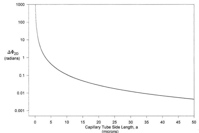
Fig. 1. Graph of expected change of phase as a function of constriction side length,  $a$ .
