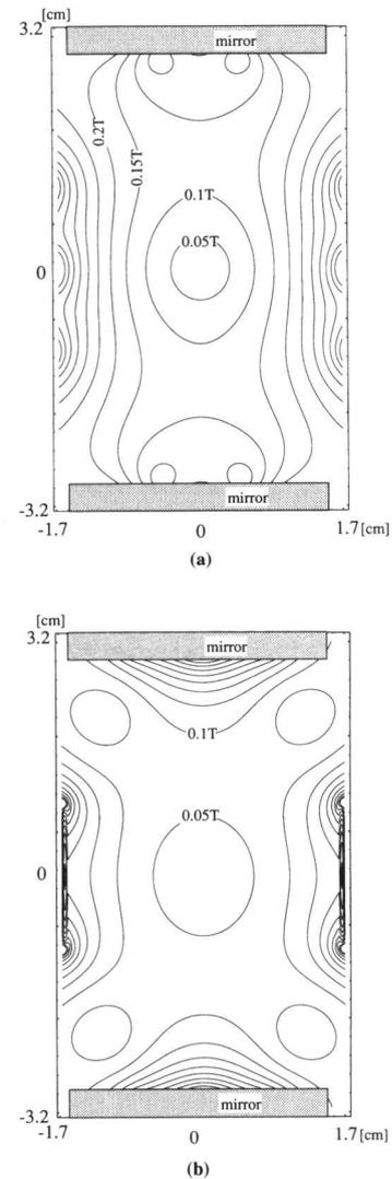
Fig. 3. The magnetic isobar in the cross section of the guide tube.
