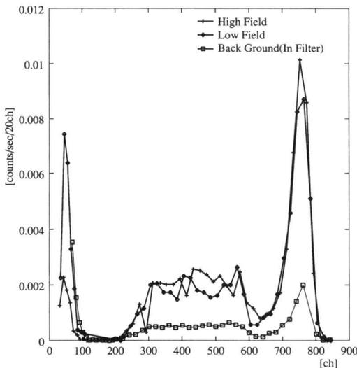
Fig. 6. The energy spectrum of detected neutrons for the high field configuration, the low field configuration, and the back ground counting.
