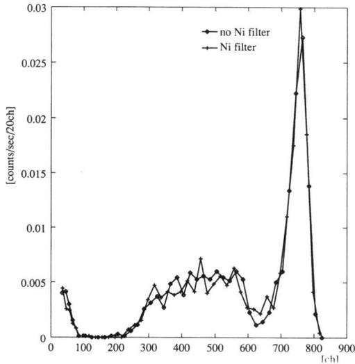
Fig. 5. The pulse-height spectra of neutron detector.
