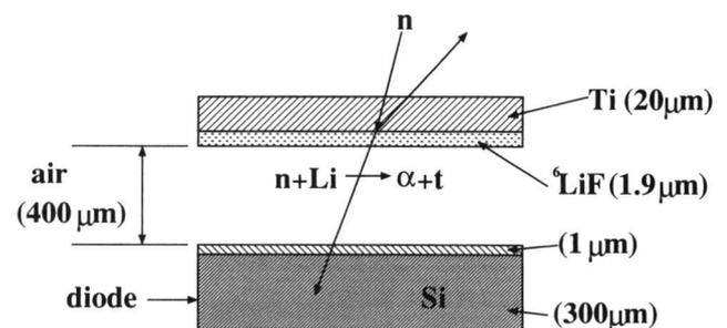
Fig. 4. Fine geometry of the detector.
