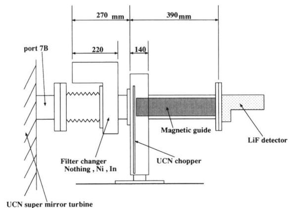
Fig. 1. Neutron magnetic transportation system.
