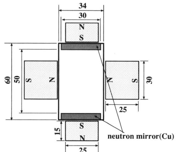
Fig. 2. The cross section of the magnetic neutron guide tube. Length of the tube is 30cm.
