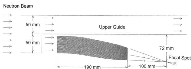
Figure 1. A schematic of the neutron bender/focuser being constructed for PGAA application.
