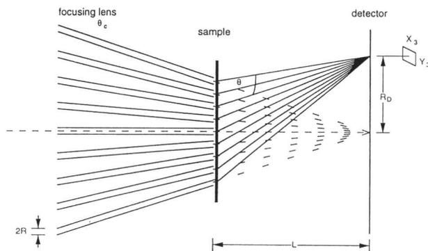
Figure 5. A schematic showing the experimental arrangement of a focusing guide small-angle neutron scattering experiment.
