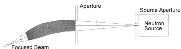
Figure 3. A schematic of a capillary optic used to focus neutrons directly from a source using a small source aperture.
