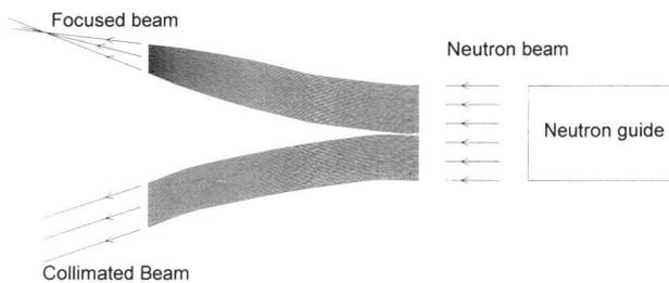
Figure 6. A schematic for a neutron beam splitter which creates both a focusing beam and a collimated beam from a single input.
