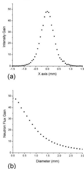
Figure 2. Simulated intensity distribution (a) normalized to the incident beam, and (b) the gains in neutron flux summed from areas of different diameters at the focus.
