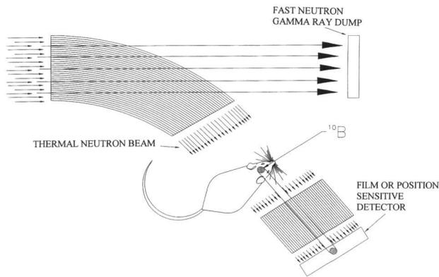
Figure 4. A schematic showing the use of a capillary optics for neutron radiography of  $^{10}\text{B}$  imaging.
