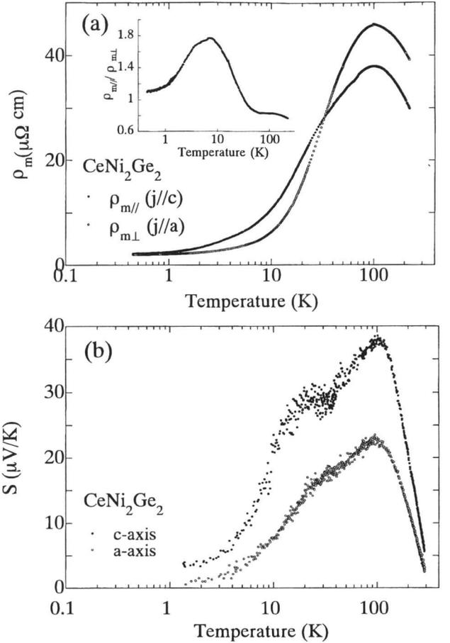
Fig. 3 (a) Temperature dependence of the magnetic resistivity  $\rho_m$ , where  $\rho_m = \rho_{\text{CeNi}_2\text{Ge}_2} - \rho_{\text{LaNi}_2\text{Ge}_2}$ . The inset show the anisotropy of the magnetic resistivity  $\rho_m(j//c)/\rho_m(j//a)$ . (b) Temperature dependence of the thermopower.
