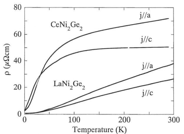
Fig. 1. Temperature dependence of electrical resistivity  $\rho$  of CeNi<sub>2</sub>Ge<sub>2</sub> and LaNi<sub>2</sub>Ge<sub>2</sub> single crystals.
