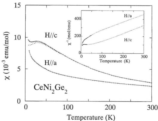
Fig. 4 Temperature dependence of the magnetic susceptibility  $\chi$  of CeNi<sub>2</sub>Ge<sub>2</sub> single crystal. The dotted line is the corrected susceptibility  $\chi_c$ ;  $\chi_c = \chi - C_0/T$ . The Curie constant  $C_0$  in the correction term is estimated from the fitting below 10 K. The inset shows the inverse of the susceptibility.
