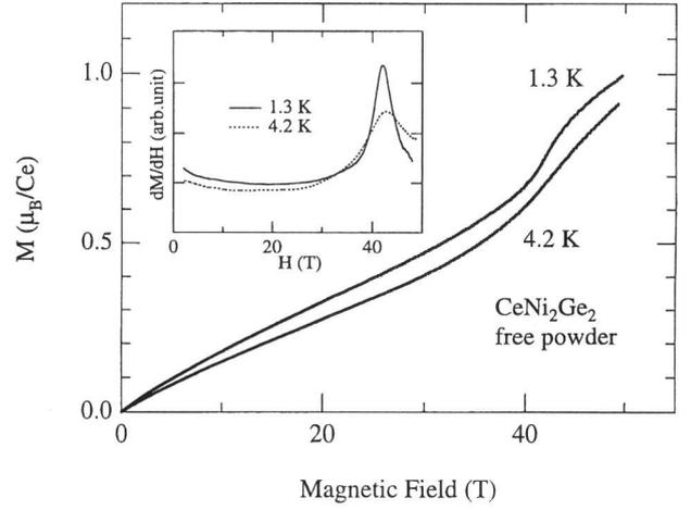
Fig. 5 Field dependence of the magnetization  $M$  of CeNi<sub>2</sub>Ge<sub>2</sub> free powder. The inset shows the differential magnetization  $dM/dH$ .
