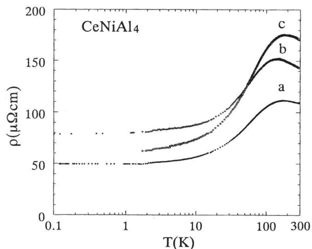
Fig.1. The  $\ln T$  dependence of the electrical resistivity of the single-crystal CeNiAl<sub>4</sub> on the a, b and c axes.
