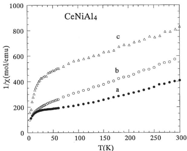
Fig.2. The temperature dependence of the magnetic susceptibility of the single-crystal CeNiAl<sub>4</sub> in the magnetic fields parallel to a, b and c axes.
