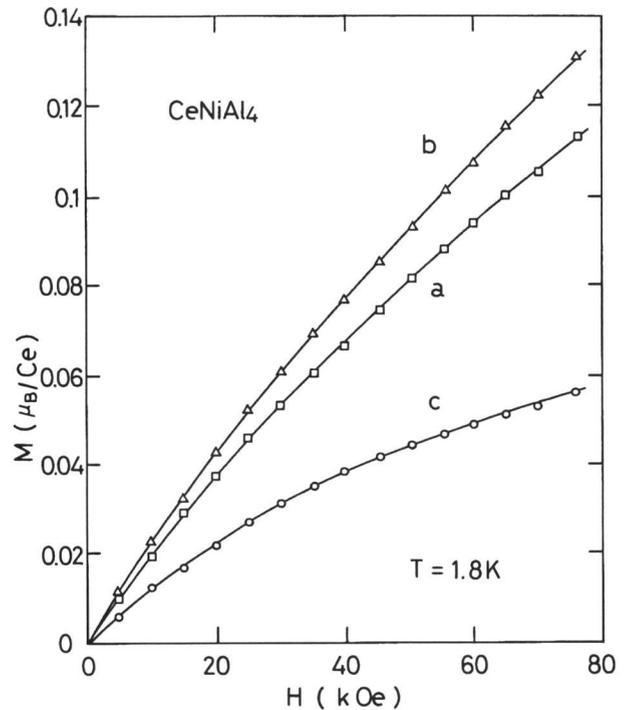
Fig.3. Magnetization process of the single-crystal CeNiAl<sub>4</sub> at 1.8K in the fields parallel to a, b and c axes.
