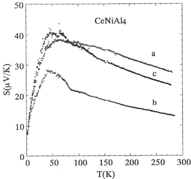
Fig.6. The temperature dependence of the thermoelectric power of single-crystal CeNiAl<sub>4</sub> on a, b and c axes.
