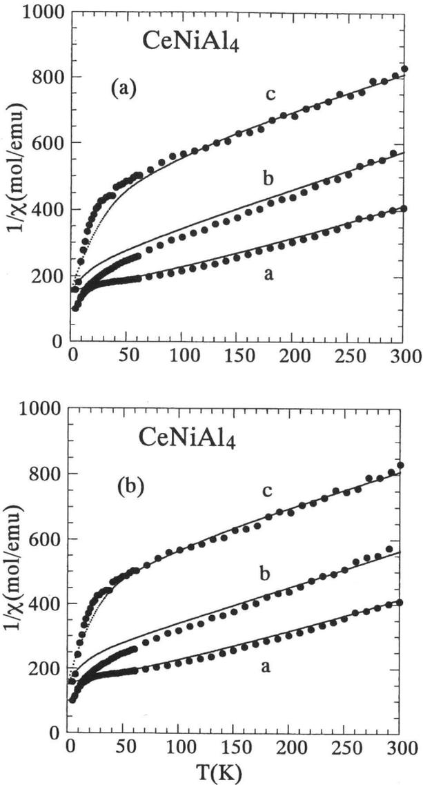
Fig.8. The temperature dependence of the reciprocal susceptibility of the single-crystal CeNiAl<sub>4</sub> in the magnetic fields parallel to a, b and c axes. Thin lines are the calculated ones using the parameters of set 1 in (a) and set 2 in (b). See text.
