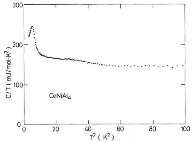
Fig.4. Specific heat divided by  $T$  vs.  $T^2$  of CeNiAl<sub>4</sub>.
