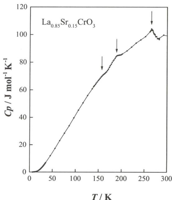
Fig.4. Temperature dependence of the heat capacities of  $\text{La}_{0.85}\text{Sr}_{0.15}\text{CrO}_3$ . The arrows indicate the temperatures at which anomalies have been found.
