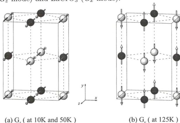
Fig.2. Magnetic structures for  $\text{La}_{0.95}\text{Sr}_{0.05}\text{CrO}_3$ : (a)  $G_z$  mode (at 10 K and 50 K); (b)  $G_y$  mode (at 125 K).
