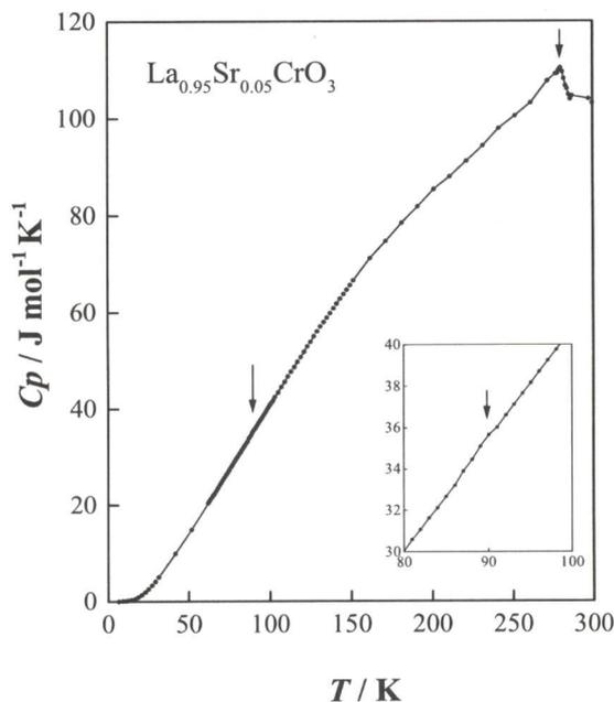
Fig.3. Temperature dependence of the heat capacities of  $\text{La}_{0.95}\text{Sr}_{0.05}\text{CrO}_3$ . The arrows indicate the temperatures at which anomalies have been found.
