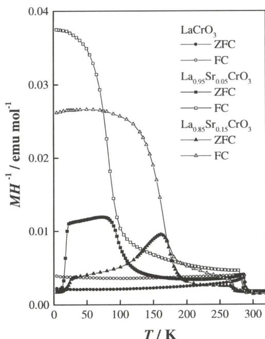
Fig.1. Temperature dependence of magnetic susceptibilities for  $\text{La}_{1-x}\text{Sr}_x\text{CrO}_3$  ( $x = 0, 0.05$  and  $0.15$ ) measured after zero field cooling (ZFC) and field cooling (FC).
