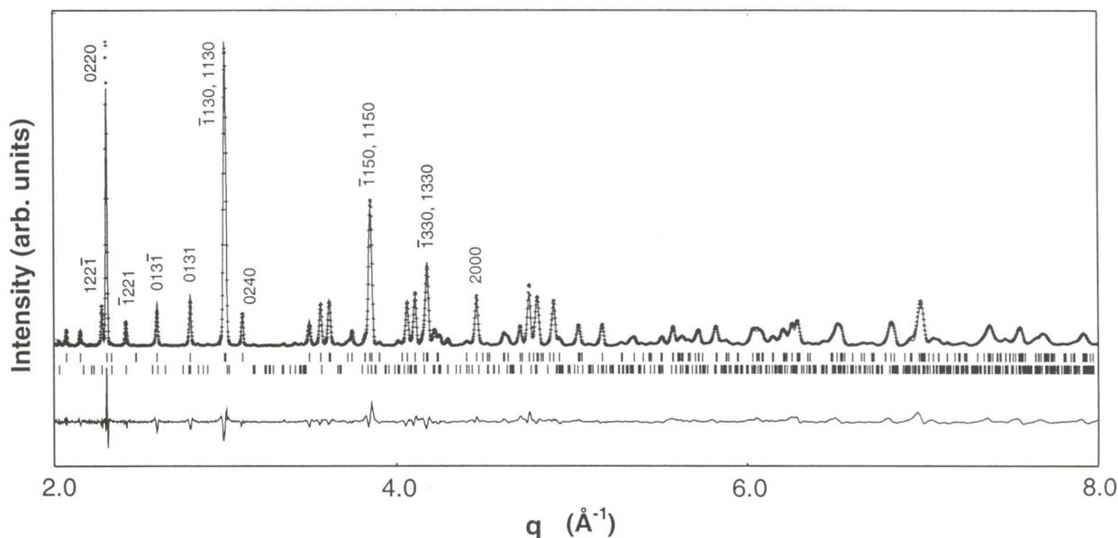
Fig.1. Observed, calculated and difference time-of-flight neutron diffraction patterns for  $(\text{Ca}_{0.565}\text{Y}_{0.435})_{0.82}\text{CuO}_2$  measured at 4 K. Short vertical lines below the pattern indicate the peak positions of main (upper) and satellite (lower) reflections for the two subsystems.
