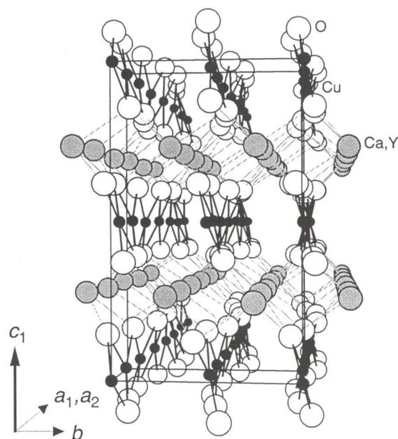
Fig.2. The modulated crystal structure of  $(\text{Ca}_{0.565}\text{Y}_{0.435})_{0.82}\text{CuO}_2$  at 4 K viewed perspectively from the  $a$ -axis.
