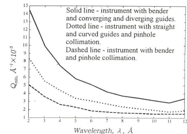
Fig.2.  $Q_{min}$  for three kinds of SANS instruments.
