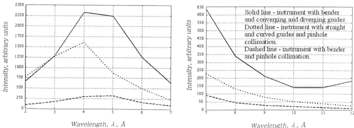
Fig.1. Neutron intensity flux for three kinds of SANS instruments.
